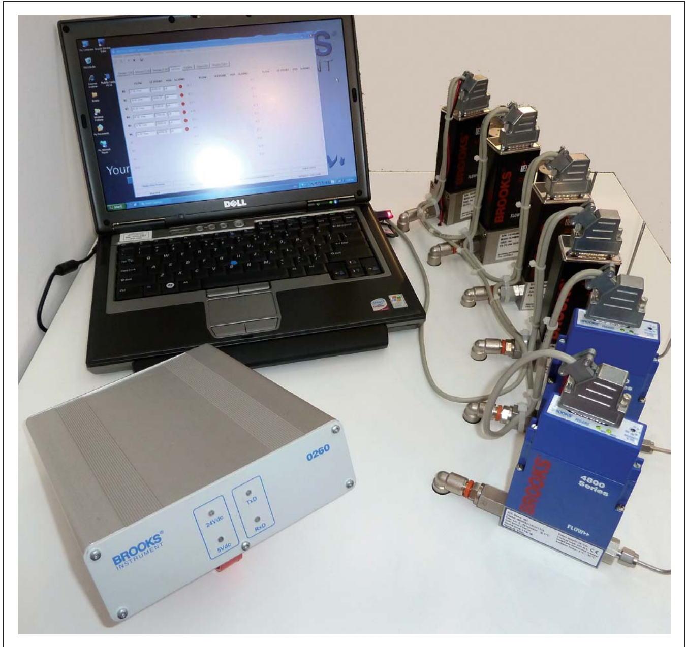
Figure 1.2 PC with Brooks® 0260 Secondary Electronics and Devices
