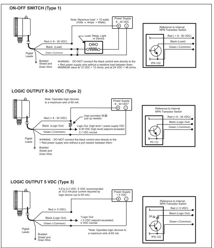
Figure 2-2 IPS122 Wiring Diagrams
