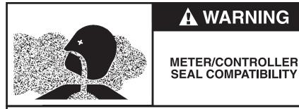
Products in this manual may contain metal or elastomeric seals, gaskets, O-rings or valve seats. It is the "user's" responsibility to select materials that are compatible with their process and process conditions. Using materials that are not compatible with the process or process conditions could result in the Meter or Controller leaking process fluid outside the pressure boundary of the device, resulting in personnel injury or death.
