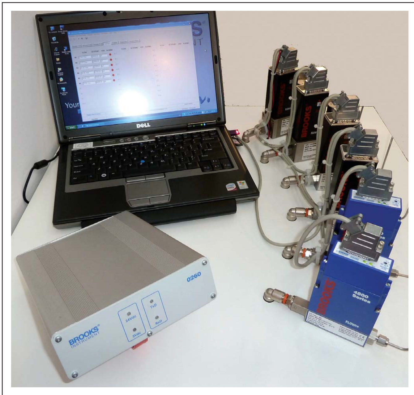
Figure 1.2 PC with Brooks® 0260 Secondary Electronics and Devices
